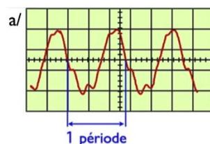
$$T_1 = 2,75 \text{ div} \times 1 \text{ ms/div} = 2,75 \text{ ms}$$
