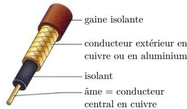
FIG. 2 – Le câble coaxial.
